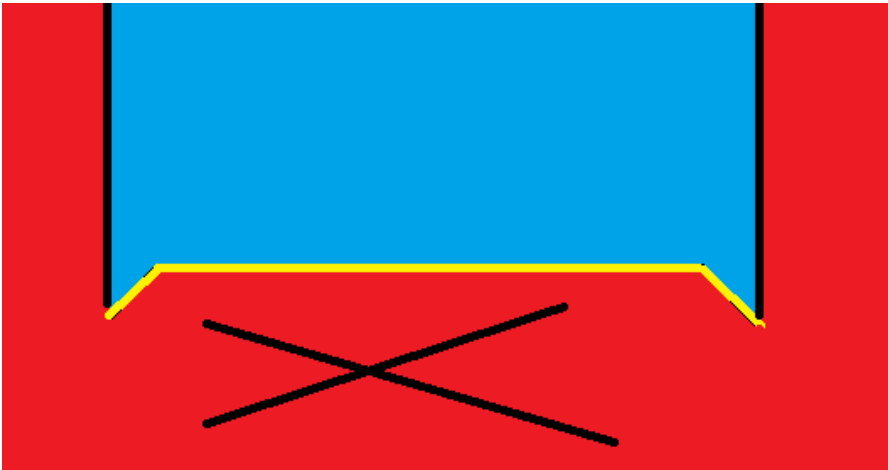
the image above illustrates an "Above", boundary, the red part is not included in the boundary, the blue part is included, the model is in yellow.
