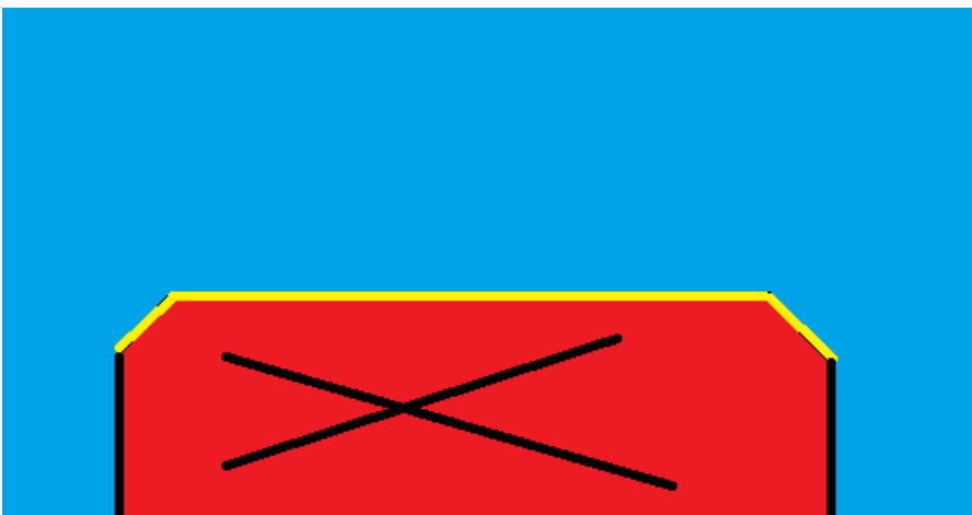
the image above illustrates a "Not below", boundary, the red part is not included in the boundary, the blue part is included, the model is in yellow.
