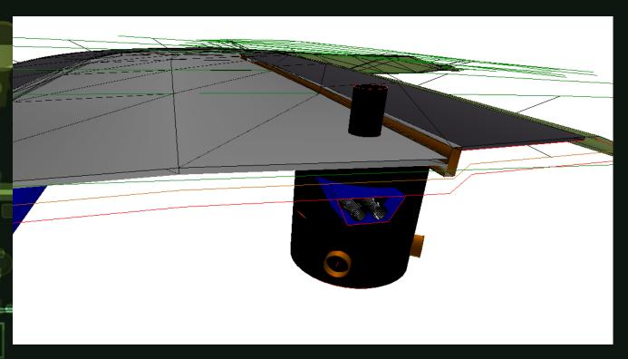
Cross sections calculation – result ends up as machine guidance and solids for export to BIM systems and for volumes.
