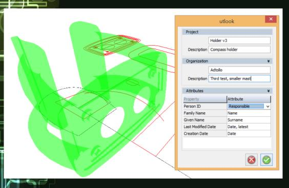
Import and export functions for IFC and CityGML, with an automatic connection between metadata and attributes
