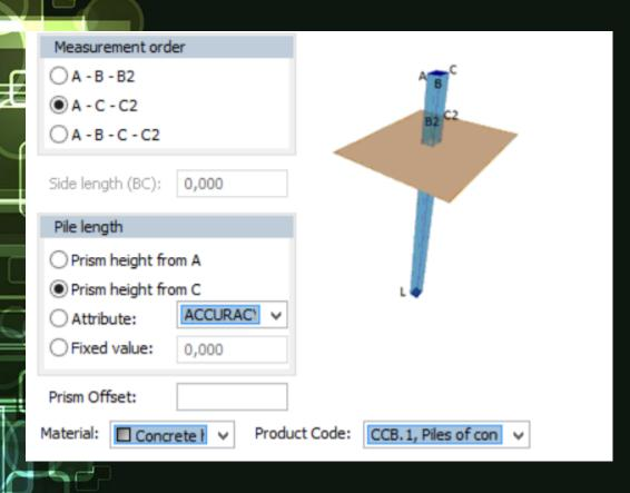
Measurement of pile, measure 2-3 corners, along one of the corners, enter length
