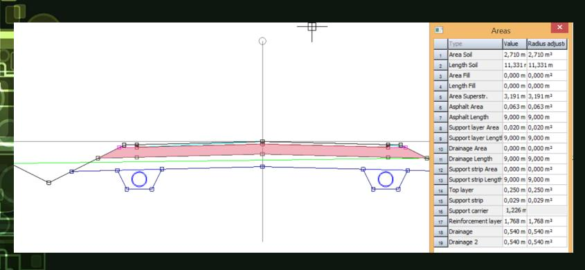
Cross sections calculation – result ends up as machine guidance and solids for export to BIM systems.
