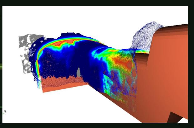
Comparisons of a point cloud vs a solid model.
